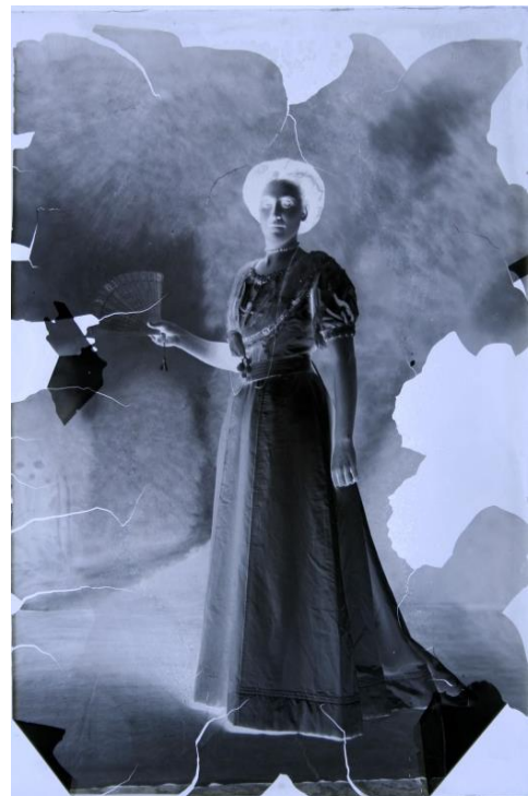
The damage on the glass plate negative (above) occurs when the gelatine emulsion swells and contracts in response to changes in humidity. The emulsion eventually lifts completely off the glass base causing large areas of image loss.
