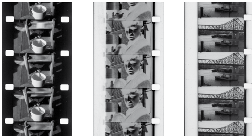
Left to right: Reversal (camera original positive, solid black edge), Negative (clear edge), Print (clear edge or solid black edge depending on printing)
